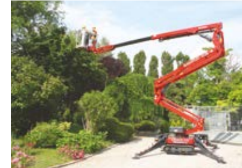
PIATTAFORME AEREE CINGOLATE Lightlift 17.75/Goldlift 14.70
